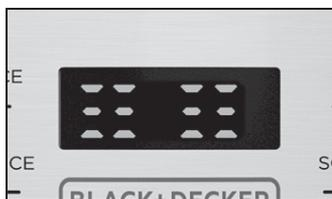
Once up to pressure, the pressure cooker will beep and the timer will start. This is also indicated by the red float valve in the elevated position.
