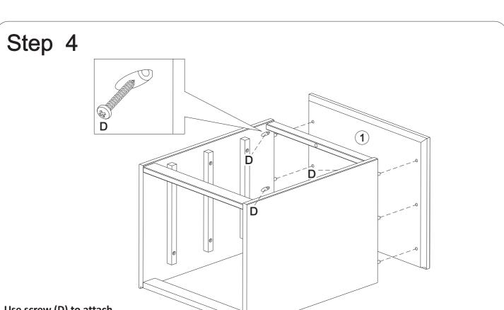
Use screw (D) to attach part (1) to body
