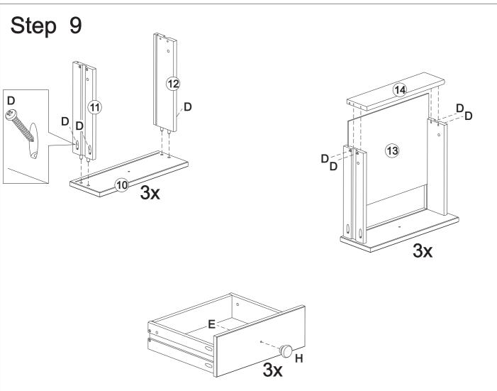
Attach parts (11,12) to part (10), insert panel (13) into groves and secure part (14) with screws(D) Insert knob (H) with screws(E).
