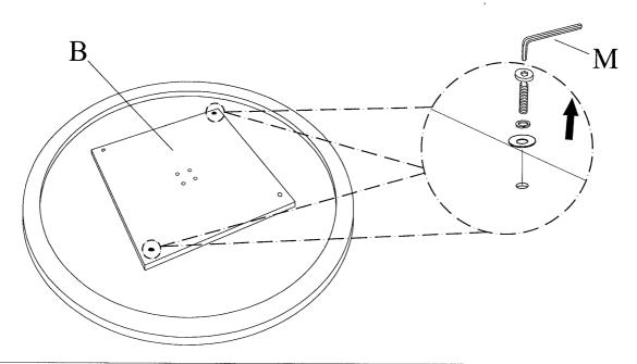
2 Align and fasten Mounting Plate (B) to Pedestal Column (C) using JCBC Bolt (E), Spring Washer (F) and Flat Washer (G) and tighten with Allen Wrench (M).
