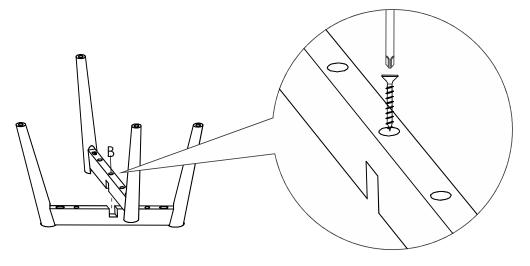
Attach part (2) to part (3) using screwdriver and screw (B)
