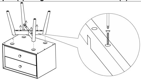
Attach legs (2,3) to body (1) USING SCREWDRIVER AND SCREW (A)
