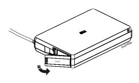
Turn off the UPS and disconnect all equipment connected to the UPS. Remove the stabilizer bracket if it is being used. Open the battery compartment door and disconnect it from the UPS.
