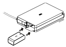
The battery connector is inside the UPS. Slide the battery into the UPS. Slight resistance will be felt as the connectors on the battery and the UPS connect.
