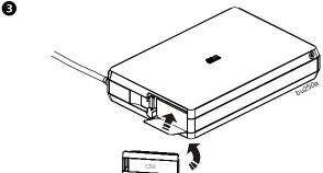
Replace the battery compartment door. Fold the battery pull tab up before closing the door.
