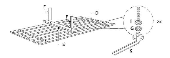
Turn the Slats (D) and place it to the Side Rail (C). Tighten the Slats (D) with CSK Screw(J) using Phillip Head Screrwdriver (Not provided).
