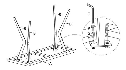
2 Attach Iron (D) to Leg (B) using Bolt (F), Spring Washer (G), Flat Washer (H) with Wrench (J).
