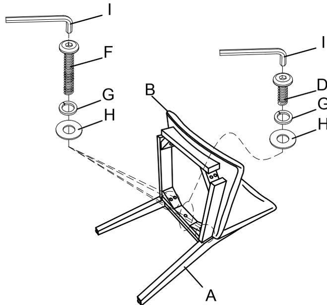
Take the Allen Key and turn the bolts until the legs are secured. **DO NOT TIGHTEN THE BOLTS COMPLETELY.** Stop when you feel you are adding force to tighten the bolts.
