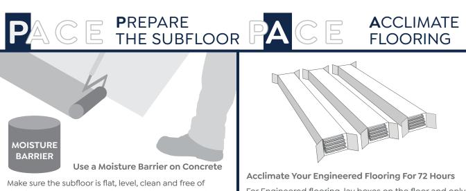
Make sure the subfloor is flat, level, clean and free of debris. New concrete must be cured for at least 60 days. Test the subfloor moisture prior to installation and apply an appropriate moisture barrier. Cali Bamboo recommends Titebond® 531+ on concrete subfloors. Although, other moisture barriers are available.
