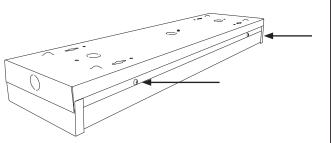
On back of fixture, use a screwdriver to knock out one of the three knockouts that corresponds to the position of your junction box – or, if connecting fixtures in-line, knock out one or both end knockout(s).
