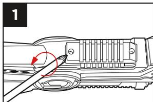
Use a screwdriver to remove the battery cover.
