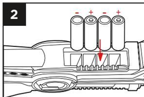
Insert 4 AA batteries. Make sure the batteries are inserted with the correct polarity.
