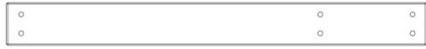
E3 | RAIL DE SOL DU NID DE CORBEAU - W4L12690 (2) | 1 3/8"x3 3/8"x33 1/2" (36x86x852)
