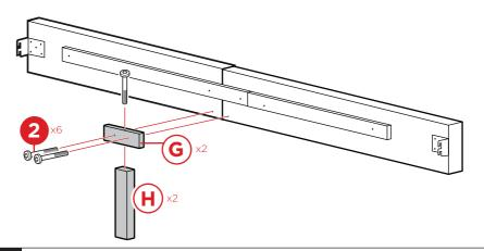
Overlap the part I center frame set, then attach four part H legs with four part 2 screws and four part 6 spring washers.
