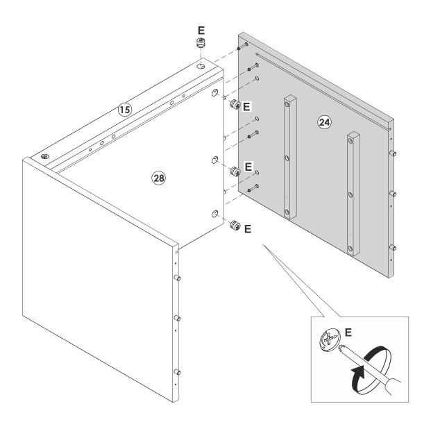
Fit part 24 to parts 28 and 15. Insert Cam lock (E) in the hole of the parts 28 and 15 and attach with Phillips head screwdriver.
