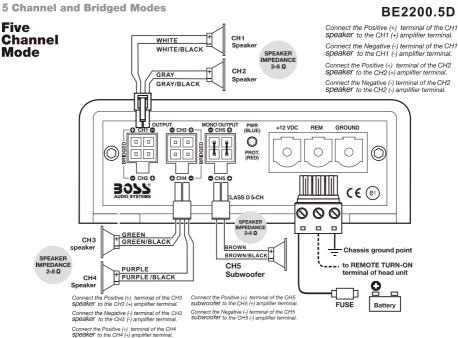
Connect the Negative (-) terminal of the CH4 speaker to the CH4 (-) amplifier terminal.
