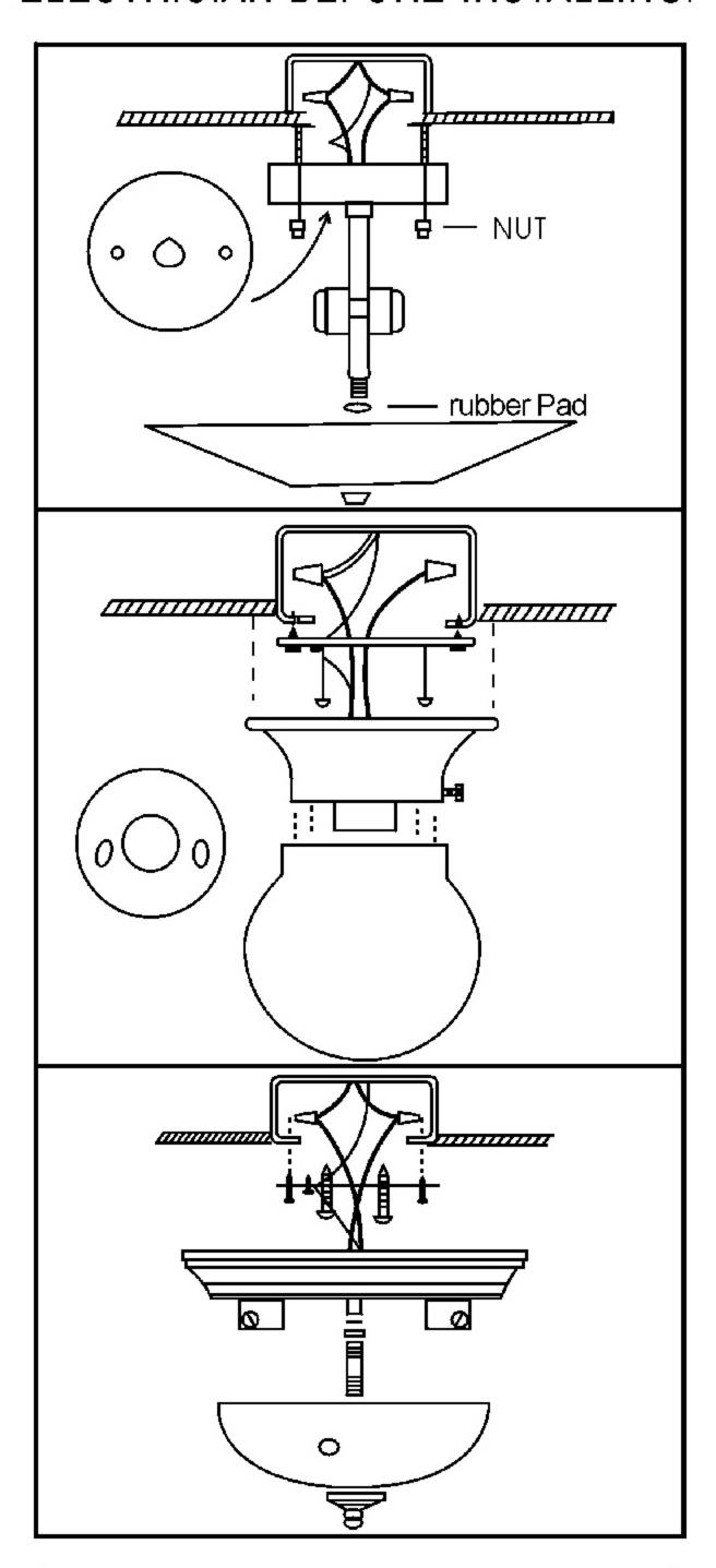
NOTE: The above diagram illustrates the installation of your new Lighting fixture. This is a representative drawing and is not intended to match the style of your fixture.
