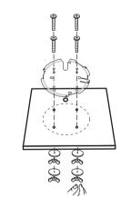
Secure the mounting bracket to the ceiling tile using pan-head screws, washers, and wing nuts, as shown on the left.
