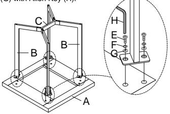
With assistance from your adult partners, turn the End Table right way up. Adjust the Pre-installed Levelers on the bottom of Leg (B) until the End Table is level with the ground.
