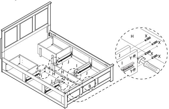
Attach Drawer Side Left (O) and Drawer Side Right (P) to Drawer Front (N) and fully tighten Cam Lock (Y) to Cam Bolt (X) using screwdriver (not provided) as image below.
