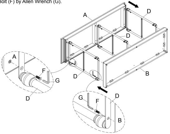
Assembly the Shelf (C) onto the Side Frame (D) and using the Bolt (F) by Allen Wrench (G).
