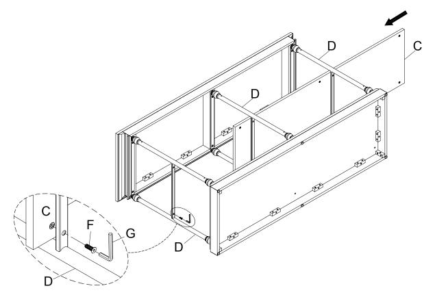
Assembly the Cross Bar (E) onto the Side Frame (D) and using the Bolt (F) by Allen Wrench (G).
