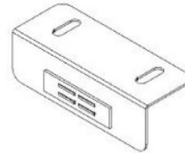
A2 SUPPORT D'AIMANT — A4M03026 (x2) 1"x1 1/4"x3 1/8" (25x31x80)
