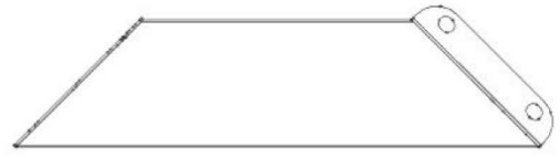
C02 ASSEMBLAGE D'ENCORBLEMENT — A4M03526 (x1) 21 13/16"x5 1/4"x2 3/4" (70x134x553.5)
