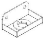
A9 ASSEMBLAGE DE SUPPORT DE TUYAU — A4M03060 (x2) 1 1/4"x1 7/16"x2 9/16" (31.5x36.5x65)
