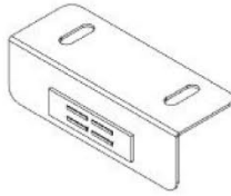
A2 SUPPORT D'AIMANT — A4M03026 (x5) 1"x1 1/4"x3 1/8" (25x31x80)
