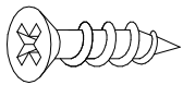
30 x 84 M3.5 x 12mm Screw M3.5 x 12mm de la vis M3.5 x 12mm el tornillo
