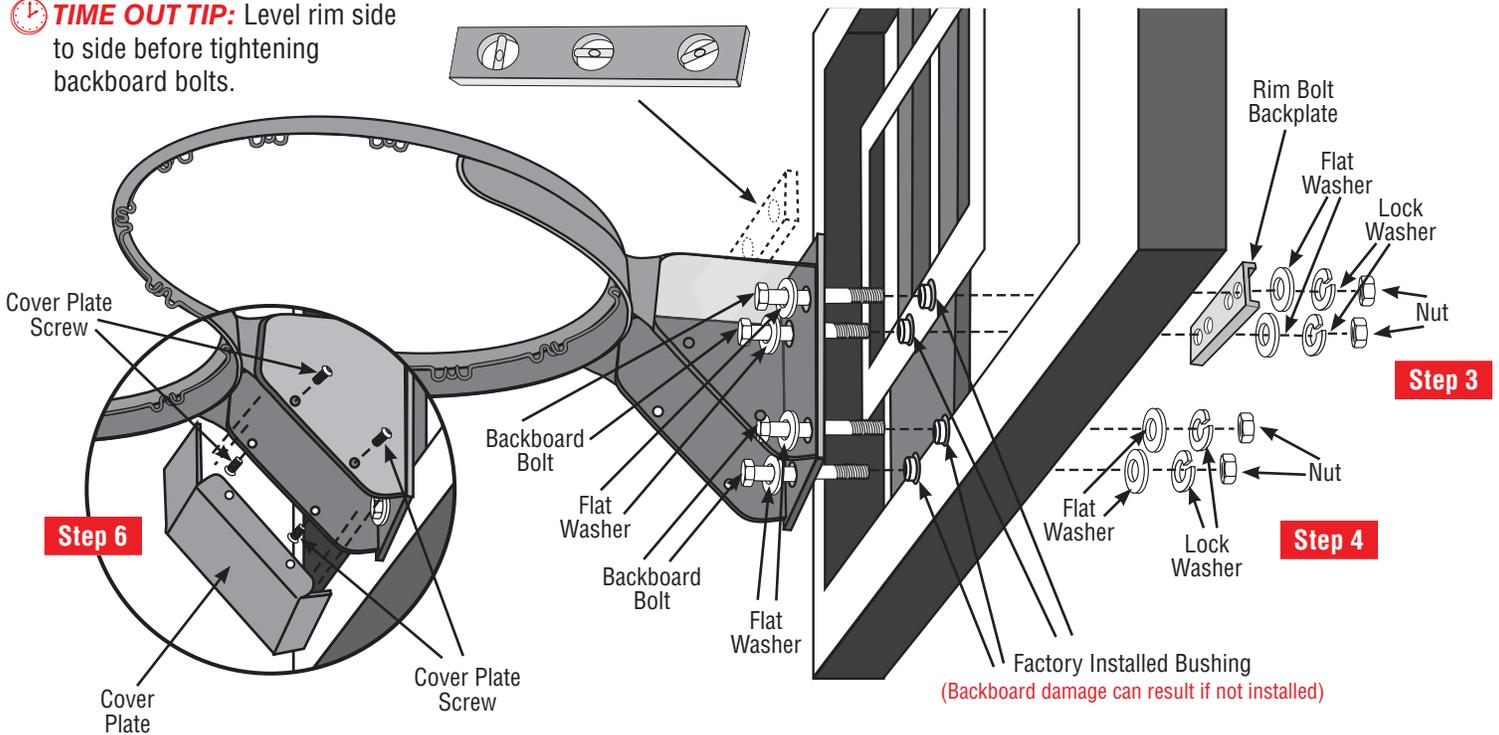
**Step 2:** If not already removed, remove cover plate screws and cover plate from rim assembly.
