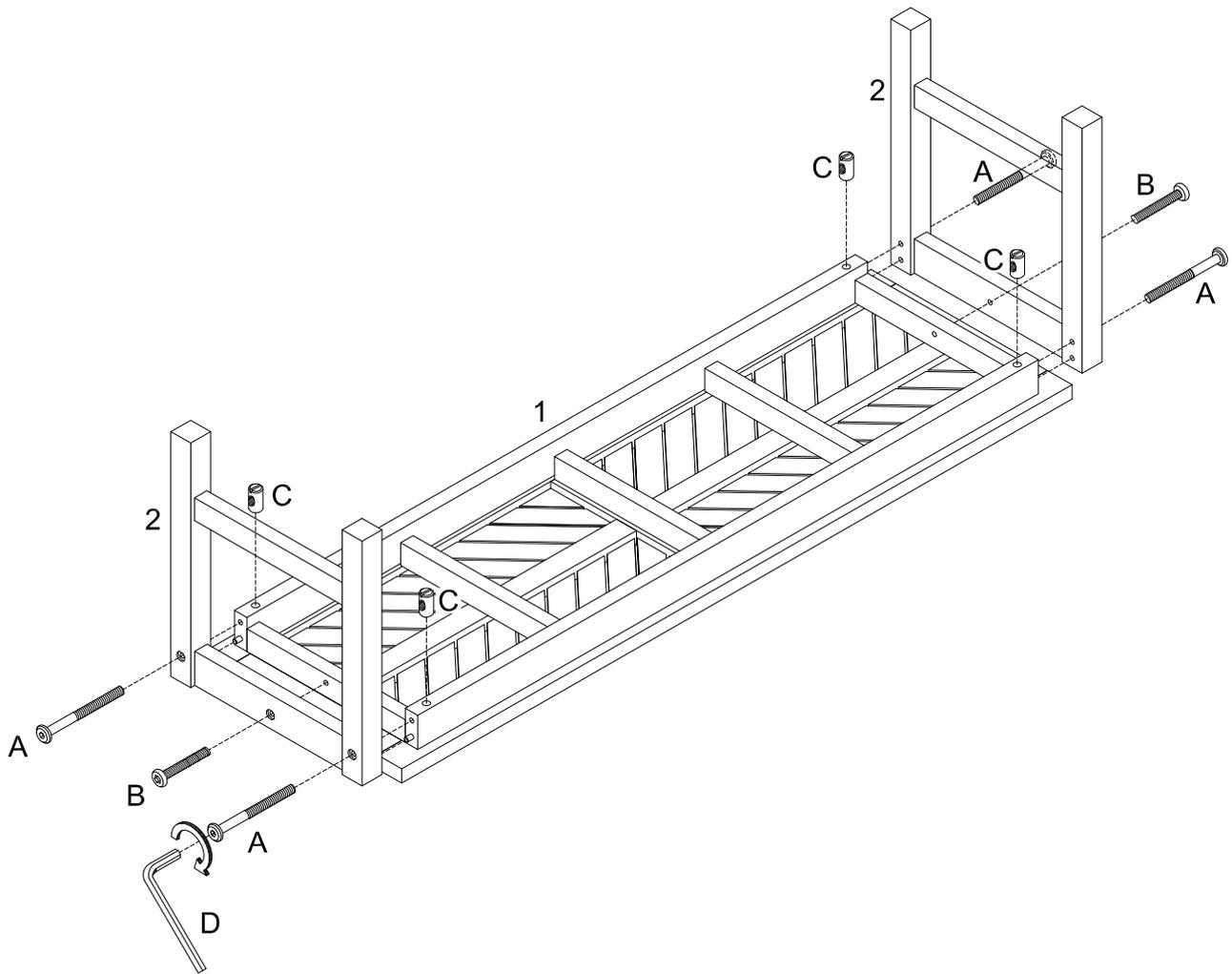
Attach part (1) to part (2) using bolt (A, B) and nut (C) with hex key (D) as per daigram.
