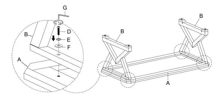
2 Attach the Shelf (C) to the Leg Frame (B) using Bolt (D), Spring Washer (E) and Flat Washer (F) with Allen Wrench (G). Fully tighten the bolts in this step.
