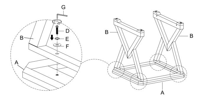
2 Attach the Shelf (C) to the Leg Frame (B) using Bolt (D), Spring Washer (E) and Flat Washer (F) with Allen Wrench (G). Fully tighten the bolts in this step.
