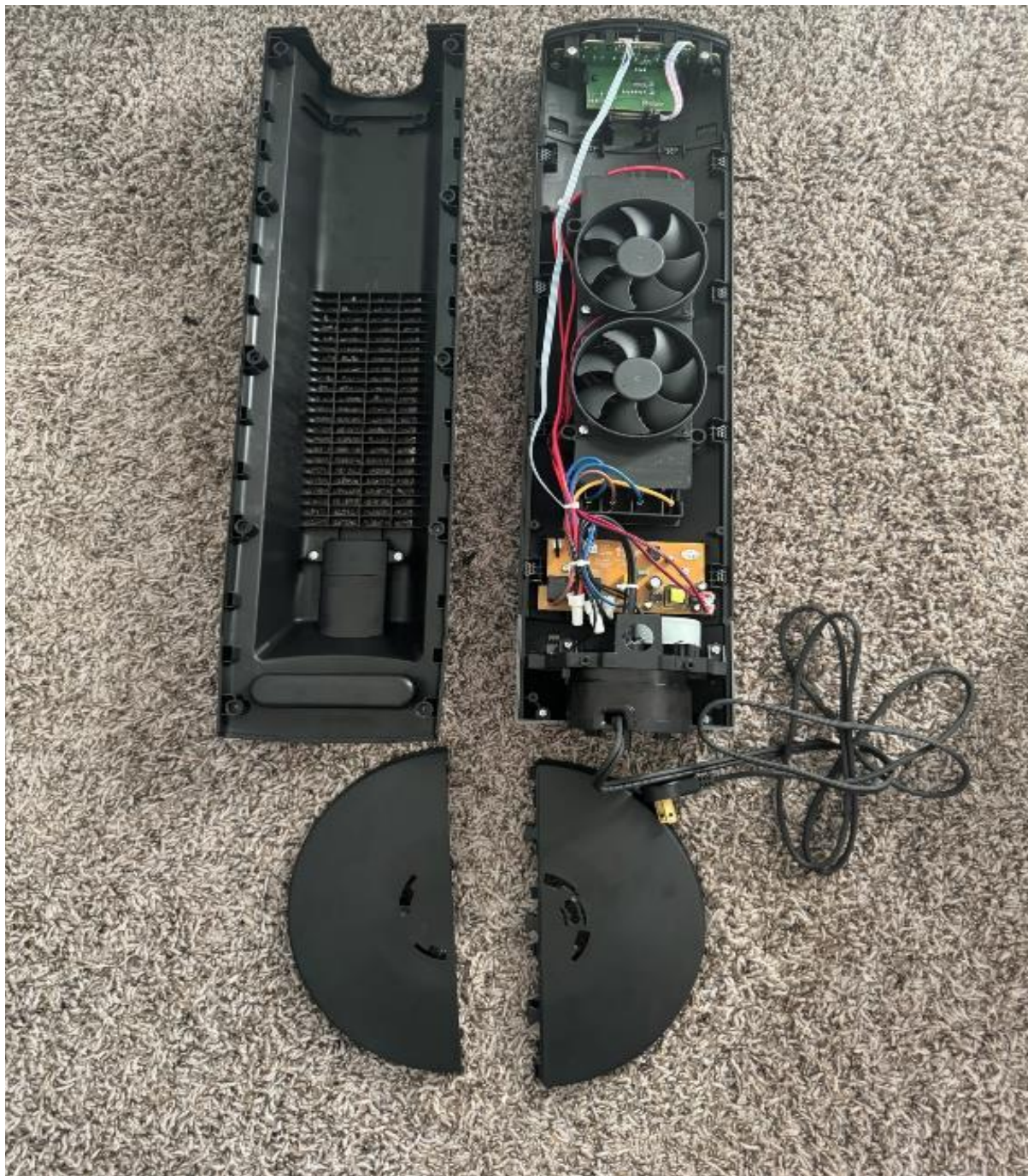
Photo 2 - Internal Overall View of CT24950
