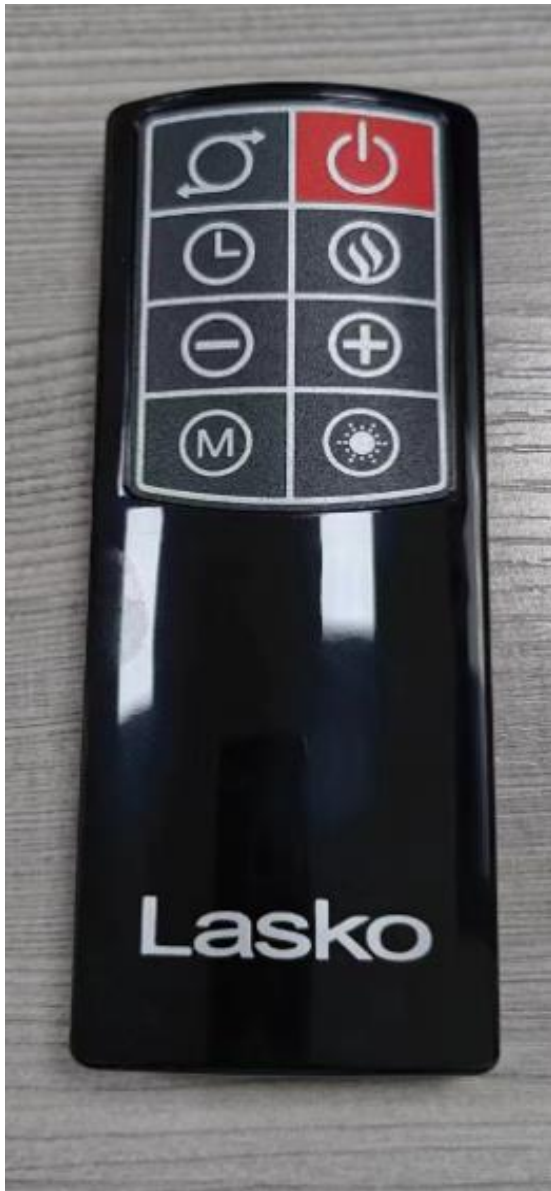
Photo 9 - Remote Control Power by AAA batteries
