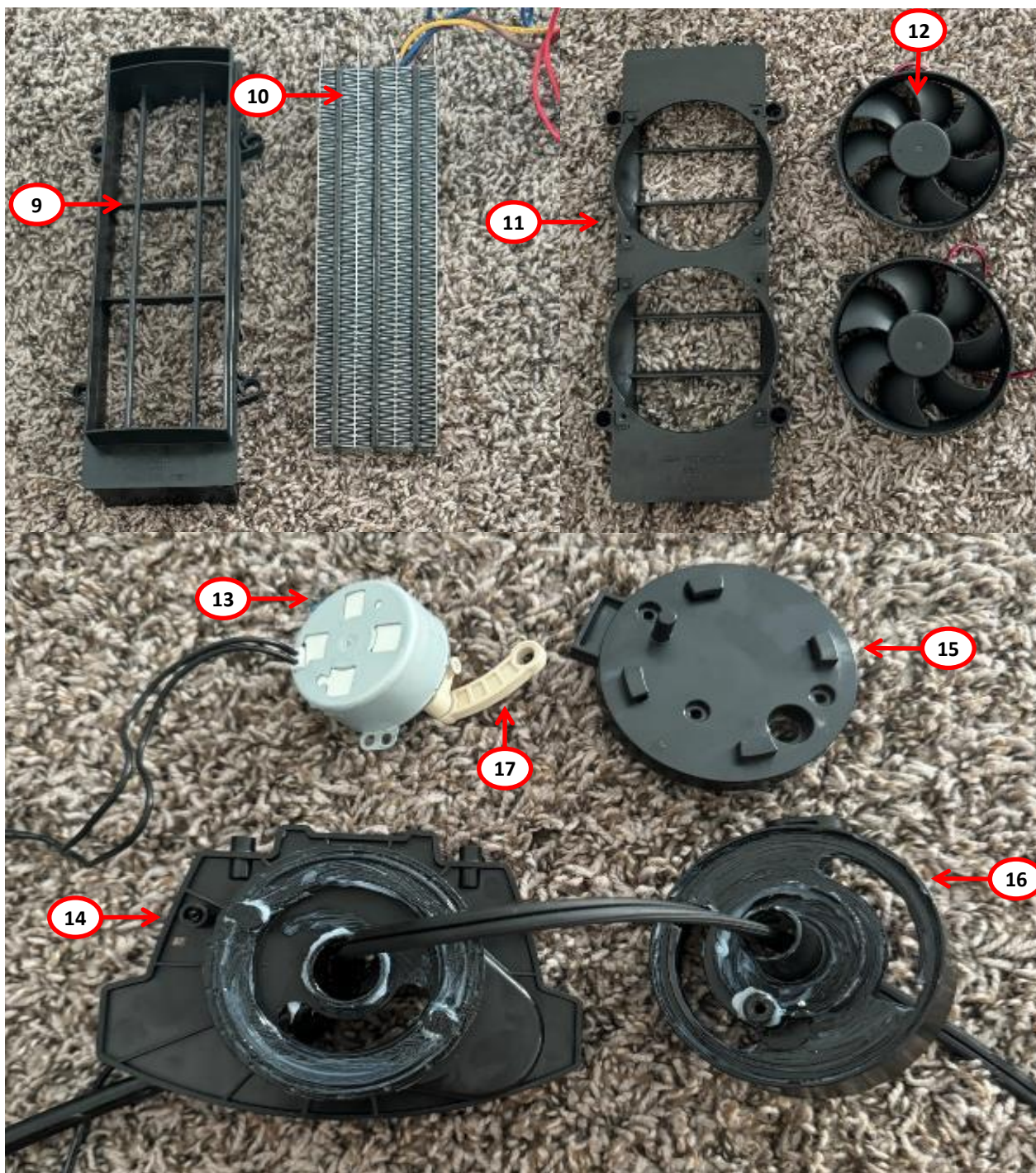
Photo 4 - Fan, Motor, Heater Assembly View of CT24950 (Also represents CS27650)
