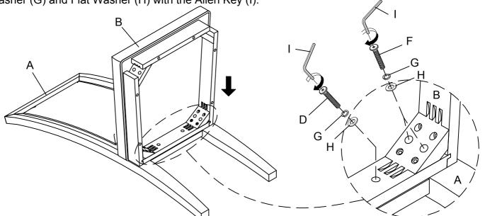
Take the Allen Key and turn the bolts until the legs are secured. DO NOT TIGHTEN THE BOLTS COMPLETELY. Stop when you feel you are adding force to tighten the bolt.
