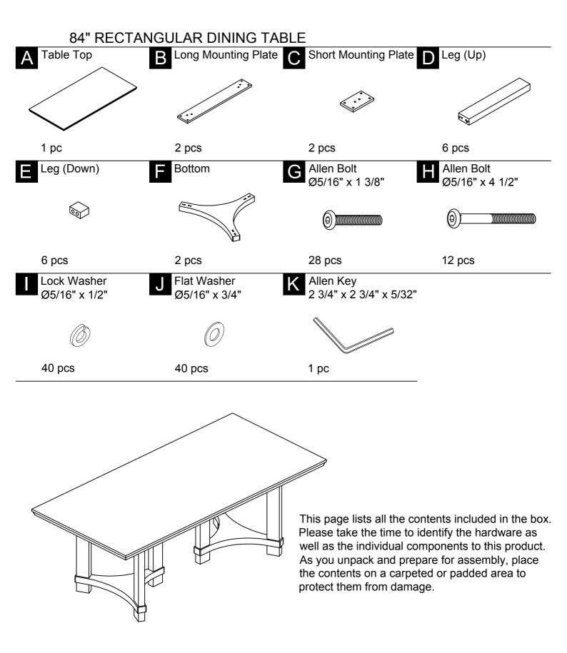
Attach the Leg (Up) (D) to the Bottom (F). Then attach the Leg (Down) (E) to the Bottom (F) using Allen Bolt (H), Lock Washer (I) and Flat Washer (J) with the Allen Key (K).
