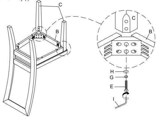
Stand the chair on an even surface and check for balance. If the chair wobbles slightly, apply downward pressure on the uneven leg and tighten the bolts to correct the imbalance. Once the chair is balanced, apply downward pressure evenly in the center of the chair and tighten all bolts, being careful not to over-tighten beyond the hole depth.
