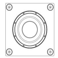
SPEAKER SPECIFICATIONSSUBB8.3Speaker Type: Powered 8" SubwooferWoofer: 8" Polypropylene Cone with Rubber SurroundPower: 150 wattsImpedance: 8 ohmsFreq. Response: 38-150 HzVoice Coil: 2" Copper-WoundPhase: 0-180°Overall Dimensions: 11.8" (299.72) x 11.8" (299.72mm) x 12.8" (325.12mm)
