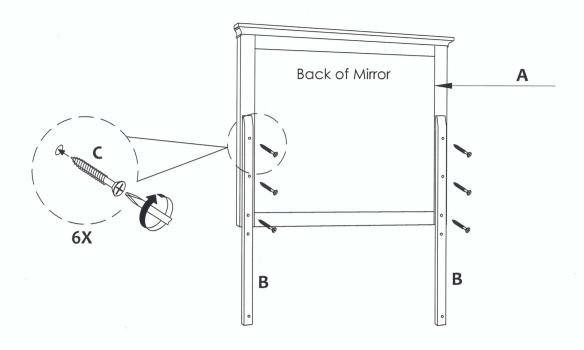
Align the Marking Line with the Mirror Back Support (B) at back of Dresser (as shown) and secure it with CSK Screw (C) using Phillips Head Screwdriver. (Not included)
