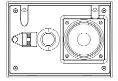
Turn the tweeter counter-clockwise to remove it from the baffle. Reinstall the new tweeter by pressing it towards the horn section of the baffle and turn it clock wise until you hear a "click".
