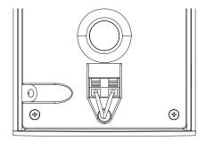
When you have installed the speaker to the wall or ceiling, then connect the speaker cable to the terminal and reinstall the front cover.
