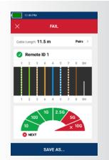
Cable test with remote attached shows remote ID number 1, length and pairing of each wire and cable performance of up to 2.5 Gb/s but failed the test due to a user-set limit of 10 Gb/s performance.
