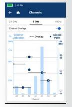
Channel test shows key information for understanding the Wi-Fi environment: number of AP's seen on and overlapping each channel and their signal strength, plus total channel utilization. Touching a channel provides details on APs on or interfering with that channel.
