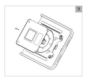
Remove the Electronics Cover from the inside of the Case.
