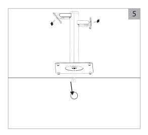
Feed the exposed wires through a hole in the table where the pillar will be installed or out the back of the pillar depending on your install requirements.
