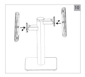
Place one or both Cases onto the Pillar head make sure to feed the cable through the center of the Case.
