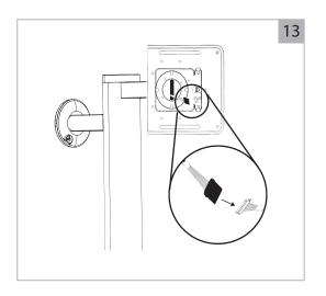
Insert the male Case Molex cable into the female Pillar Molex connector and ensure the retention cover is secured.
