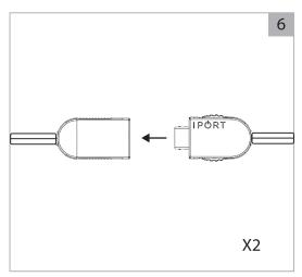
Attach the H10 Connector with the USB-C into the female H10 Connector on the Pillar System. Repeat for both connectors.
