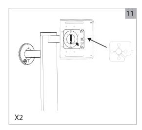
Insert the Case mounting plate into the case and over top of the Molex cable. Repeat this step for a second iPad.
