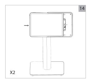
Insert the iPad into the Case ensuring the iPad is seated fully into the bottom of the Case and the USB-C connection.
