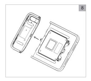
Remove the Sleeve Top From the CONNECT Case.
