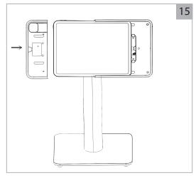
Reinstall the Case Top onto the iPad and Case making sure to fully snap the Case Top in place.
