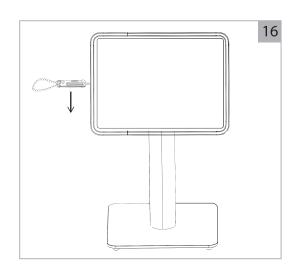
Insert the provided IPORT Security tool into top of the Case and slide towards the lock position securely locking the iPad into the Case.
