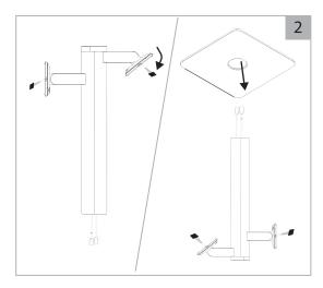
Rotate the top Mount head temporarily downward and flip the Pillar upside down to stand on its flat top. Feed the cables through the hole in the plate and rest the plate on the Pillar aligning the notch between the two parts.
