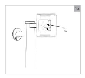
Insert the 4ea provided philips head screws into the Case mounting plate and tighten snug ensuring the case is secure to the pillar head.
