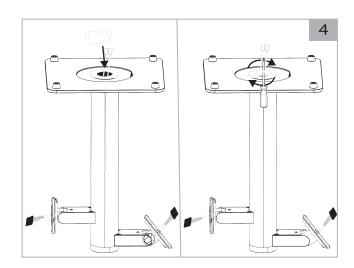
Insert the provided key wrench into the mounting nut slots and tighten by hand. Insert a screwdriver into one of the holes in the wrench to use extra leverage in tightening the nut.
