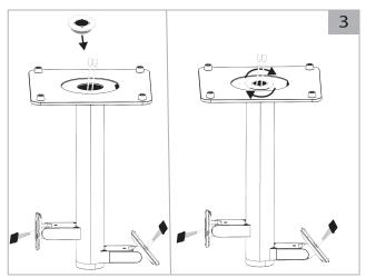
While holding the baseplate in place, feed the cables through the mounting nut. Spin the mounting nut clockwise into the pillar until it is tight.
