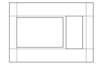
Faceplates with outlet are reversible and can be used for outlets on the left and the right.
