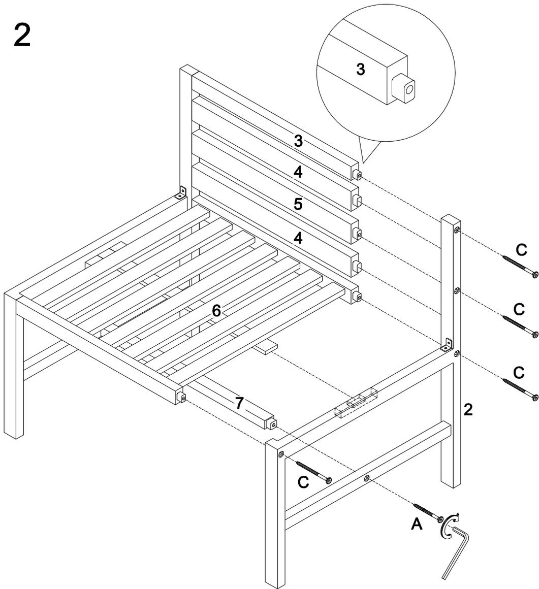
Repeat the last action as per diagram. Fully tighten all the bolts .
