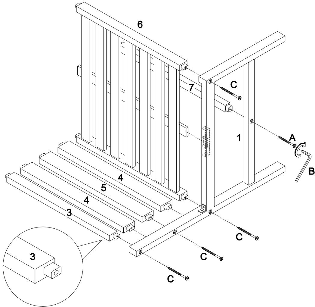
Insert part (4) into part part (1) as per diagram. Using bolt (A) insert into part (1) to part (7) ,and using bolt (C) into part (1) to parts (3,5,6) with hex key (B) as per diagram.
