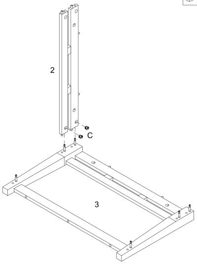
Using Cam lock(C) secure part (2) to part (3) with Philips head screwdriver as per diagram.
