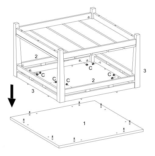
Using Cam lock(C) secure part (1) to parts (2,3) with Philips head screwdriver as per diagram.
