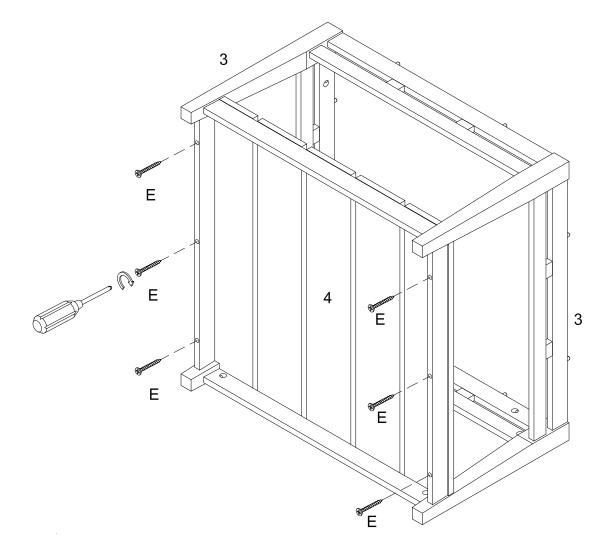
Using screw (E) attach part (3) to part (4) with Philips head screwdriver as per diagram.
