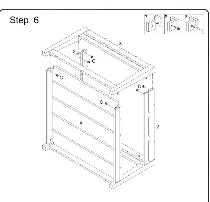
Using Cam lock(C) secure part (3) to parts (2,4) with Philips head screwdriver as per diagram.
