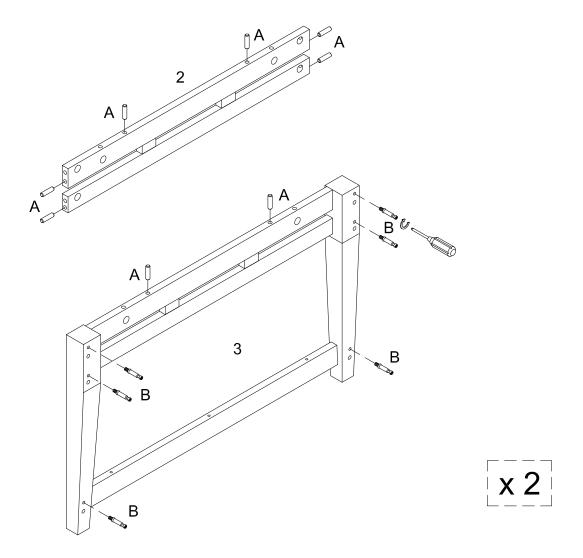
Insert wooden dowel (A) into parts (2,3), then secure cam bolt (B) into part (3) with Philips head screwdriver as per diagram.
