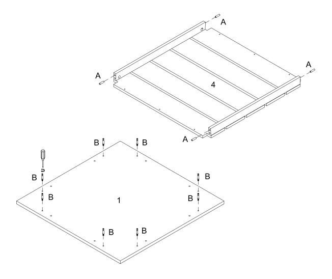
Insert wooden dowel (A) into part (4), then secure cam bolt (B) into part (1) with Philips head screwdriver as per diagram.
