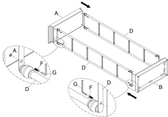
Assembly the Shelf (C) onto the Side Frame (D) and using the Bolt (F) by Allen Wrench (G).
