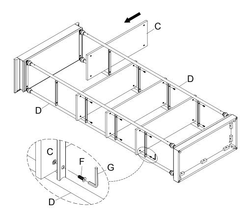
Assembly the Cross Bar (E) onto the Side Frame (D) and using the Bolt (F) by Allen Wrench (G).
