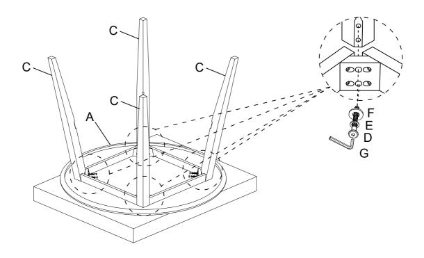
Attach Table Shelf (B) to Table Leg (C) using Bolt (D), Spring Washer (E) and Flat Washer (F) with Allen Wrench (G). Fully tighten all the bolts in this step.
