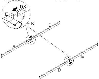
Attach the Front / Rear Support Bar (G) and Center Support Bar (F) to the Rail (D) & (E), insert the Bolt (J), turn the L-Allen Key (K) to tighten them.
