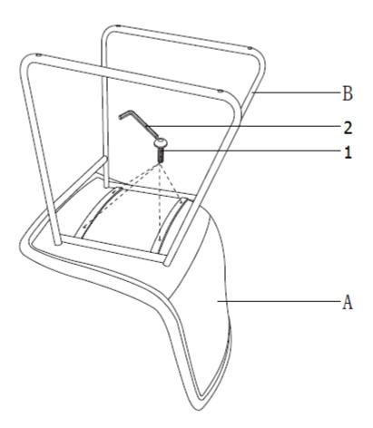
Place the Chair (A) upside down on a flat smooth surface. Attach the Base (B) to the bottom of the Chair (A) with Bolt (1). Use Allen Key (2) to tighten.
