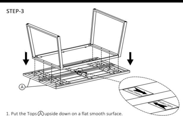
2. Attach Tops (A) to assembled Metal frame.
