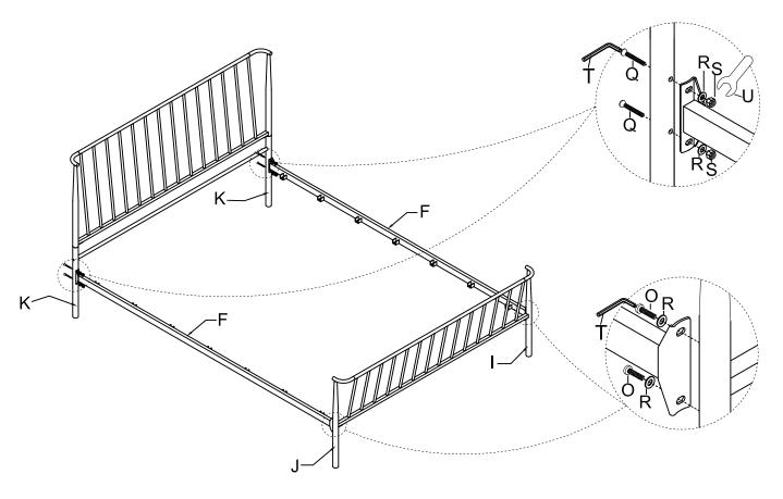
Attach the Slat (D) to the Side Rail (F).
