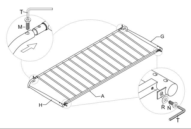
Attach the Footboard (B) to the Footboard Post (I & J) using Bolt (M & N) and Flat Washer (R) with the Allen Key (T).
