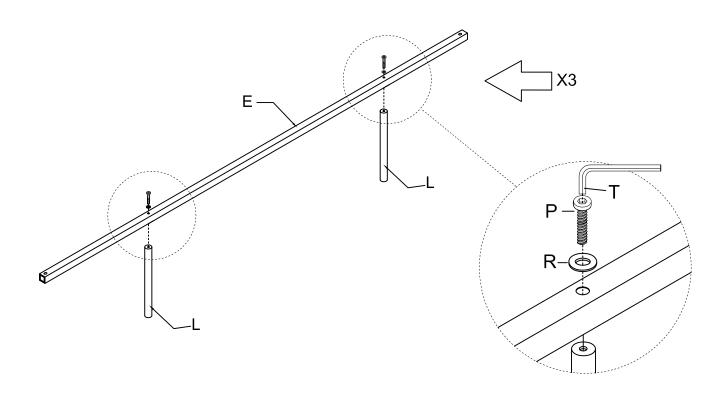
Attach the Slat (E) to the Side Rail (F) using Bolt (P) and Flat Washer (R) with the Allen Key (T).
