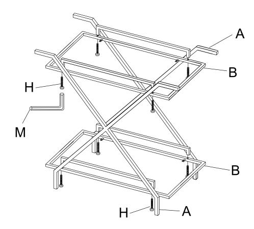
Attach Stretcher (C) to Metal Frame (B) by Bolt (H) and Allen Wrench (M) as shown.
