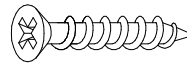
31 x 8 M3.5 x 16mm Screw M3.5 x 16mm de la vis M3.5 x 16mm el tornillo
