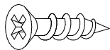
30 x 28 M3.5 x 12mm Screw M3.5 x 12mm de la vis M3.5 x 12mm el tornillo
