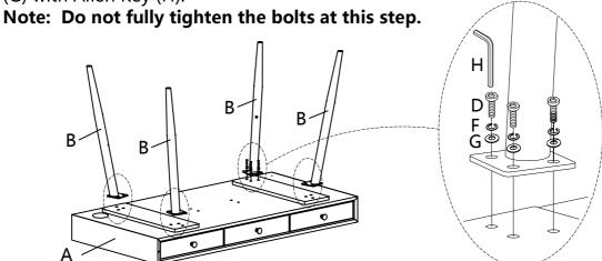
Attach Rail (C) to bottom of Top (A) using Bolt (E), Spring Washer (F), Flat Washer (G) with Allen Key (H) and attach Rail (C) to Leg (B) using Bolt (E) with Allen Key (H).
