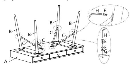
With assistance from your adult partners, turn the Desk right way up. Adjust the Pre-installed Levelers on the bottom of Leg (B) until the Desk is level with the ground.
