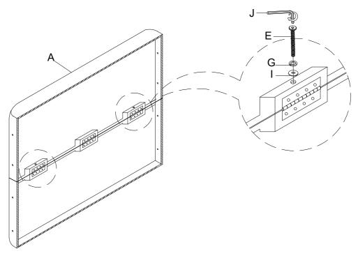
Cover H/B Piece Cloth (B) to Headboard (A). Remark: The arrow label on top of Headboard.
