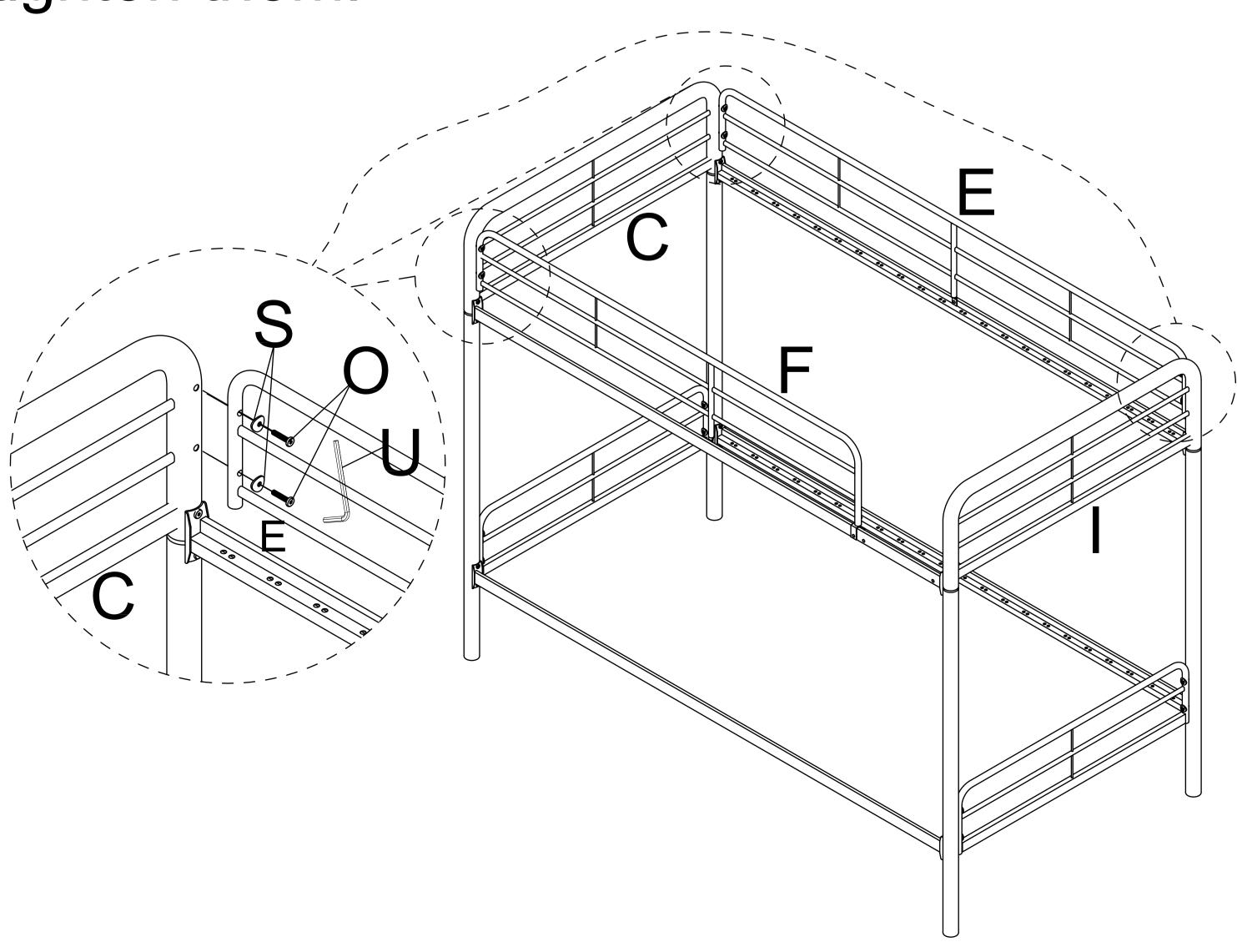
Attach the Guardrail (F) and Guardrail (E) to Upper Front Rail (H) and Upper Rear Rail (G), insert the Bolt (Q) and the Nut (T), turn the L-Allen Key (U) and the Wrench (V) to tighten them. And insert the Bolt (R), turn the L-Allen Key (U) to tighten them.
