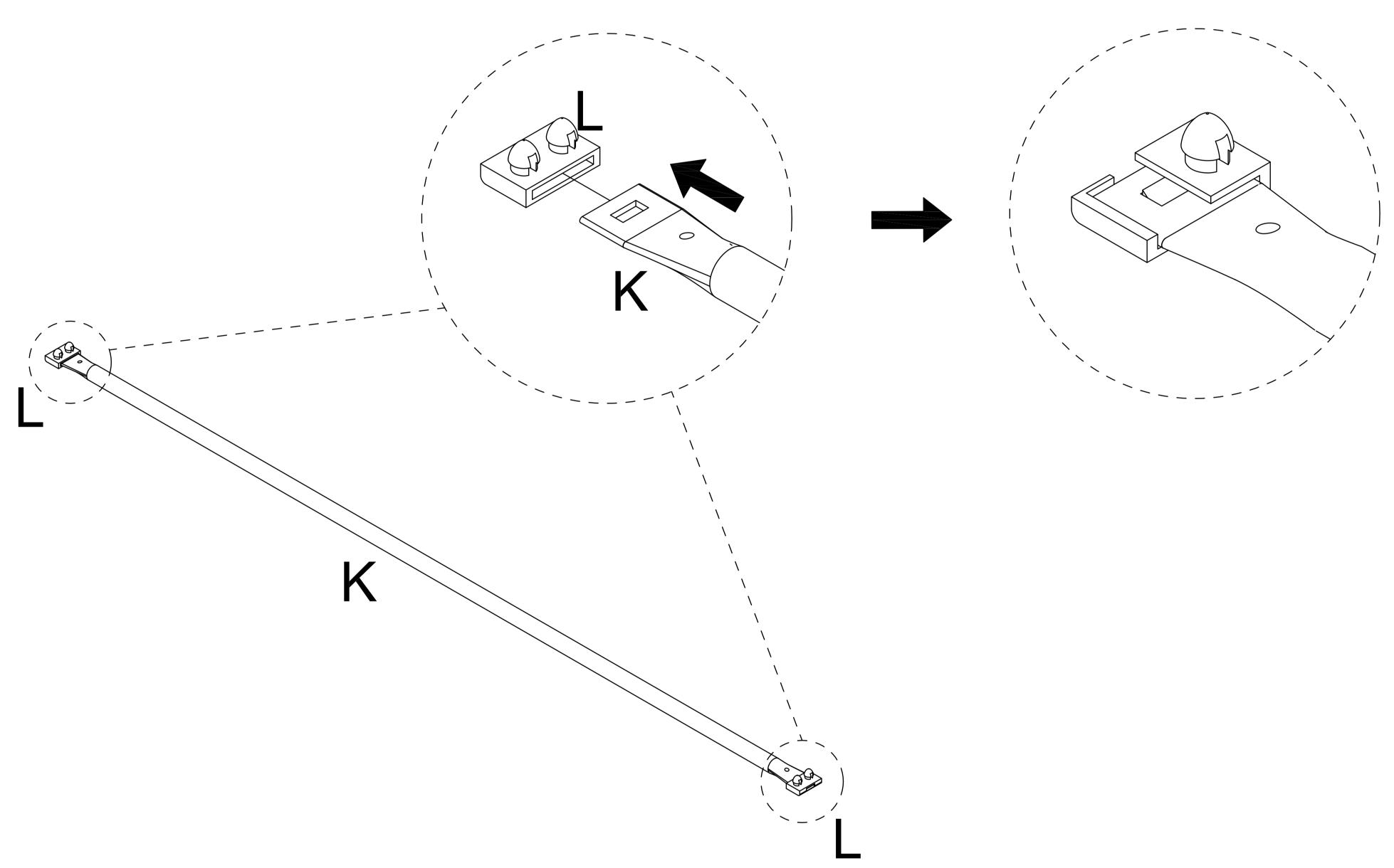
Attach the assembled Slats (K) to the upper and lower rails, insert the Slat Connector (L) into the correct holes.
