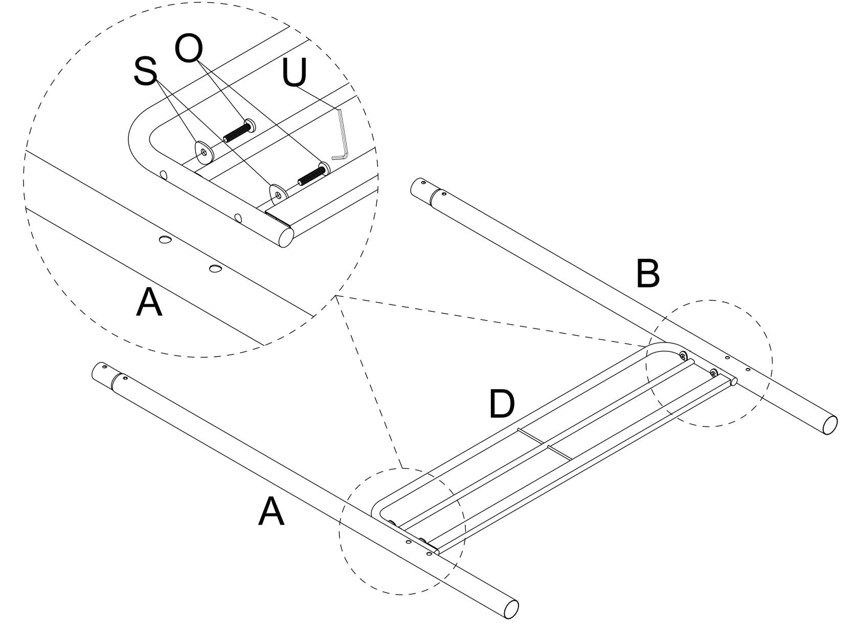
Insert the Guardrail (C) to the Post (A) and Post (B).
