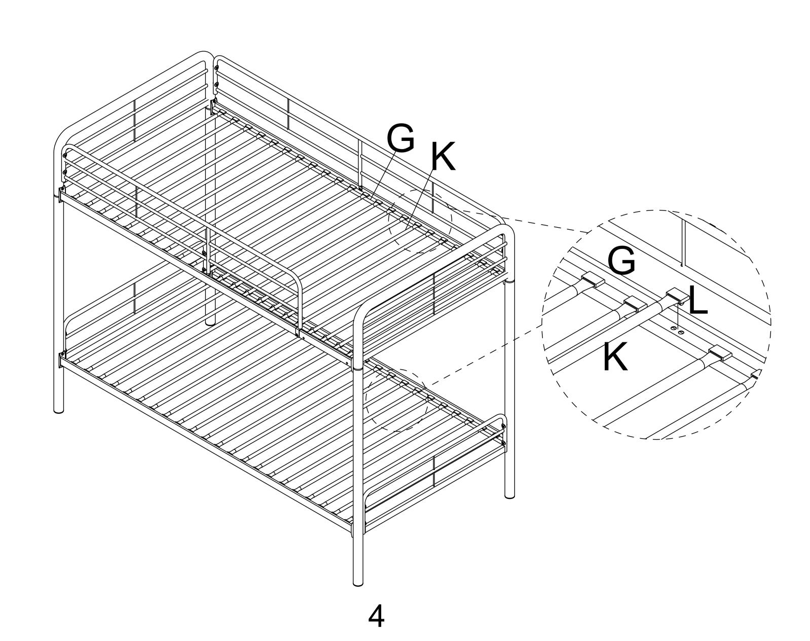
Make the Slat Spacer (N) to connect two slats as below instruction.
