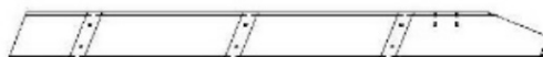
H80 MONTANT DROIT - W4L14945 (x1) 1 po x 3 3/8 po x 38 3/8 po (24 x 86 x 976)
