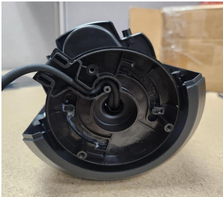
Photo 8 - Strain Relief Method
