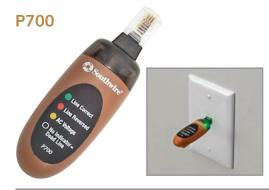
The P700 checks phone outlets - Lines 1 and 2 - for correct wiring, line reversed, AC ring voltage, and dead line conditions.
