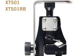
The XTS-01 Cable Stripper is made for end and mid-span terminations of 600 volt 1/0 AWG to 1000 KCMIL or outside diameters from .33"-1.284". Works on THHN, XHHW, RHH, RHW, and USE jackets.
