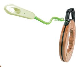
The SIMpull<sup>™</sup> Non-Conductive Tip Fish Tape has a spiral extruded polymer design that reduces the amount of effort required to push or pull the fish tape through EMT or PVC conduit. It also features a non-conductive leader.
