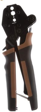
The compound leverage design delivers high crimp force with low hand force, and the near-parallel jaw action delivers precision crimps. The RCT-D1 is where power meets precision.
