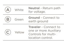
Wires are all a five inch #16 AWG stranded wire.
