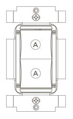
Keypad Buttons - Press the up or down button to send control data over the yellow traveler wire to a master wireless keypad dimmer or switch.
