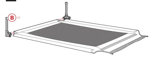
Insert two part C long frames into the legs. Route the long frames through the bed.
